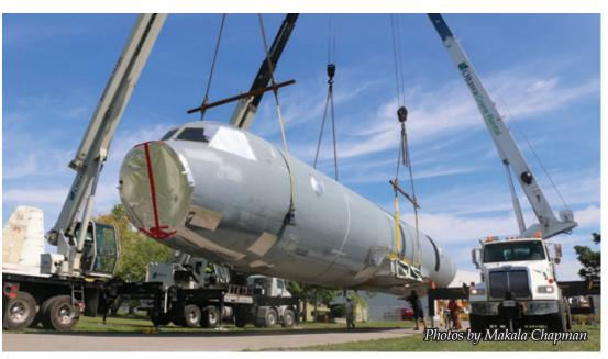
Three cranes work together to move the fuselage of the CP-140 Aurora from the bed of the tractor-trailer on Sept. 7.
