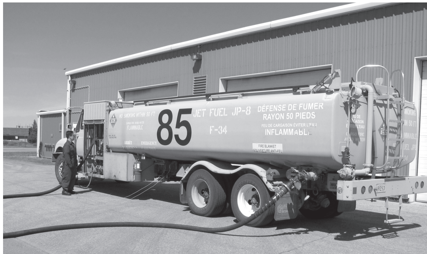
Photo by-Samuel Gillespie Corporal Rui Jiang from the Refuelling Section is performing a recirculation on one of our many refuellers in preparation for daily operations. The professional members from the Refuelling Section are on standby 24 hours a day all year round at a moment's notice.
