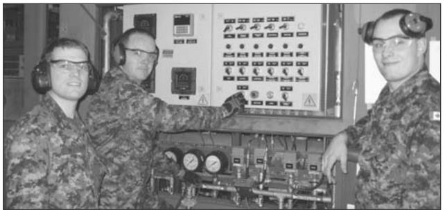
Cpl Mikhail, Cpl Connors and Cpl McManus conducting a 10-year overhaul on a 4 CES Reverse Osmosis Water Purification Unit (ROWPU). As Water, Fuel and Environment Technicians (WFE Techs) at 86 ASU, their job is to ensure that the unit is stripped, painted and mechanically tested so that our troops in the field get clean, pure water, free from contaminants. This ROWPU is a 1 Cdn Air Div deployable asset used on deployment in any location where fresh water is required.
